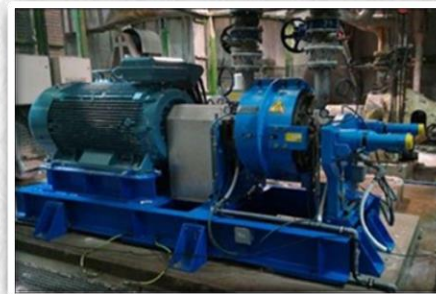
Paper Refiner Improvement by Papillon refiner CS380 (Cylindrical)
